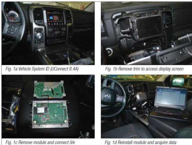
Figures 1a – 1d In-vehicle data acquisition of 2015 RAM 1500 UConnect 8.4A
